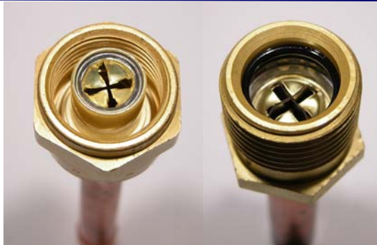
Clean and Lubricate Quick Connect Couplings
