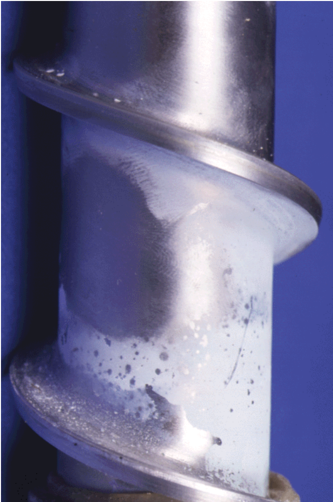
Extreme Scale Build Up on Evaporator Wall
