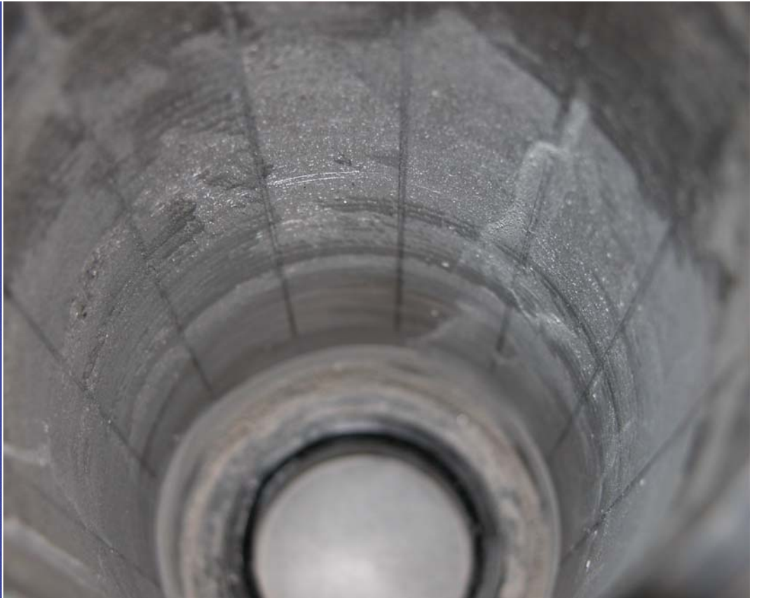
Extreme Scale Build Up on Evaporator Wall
