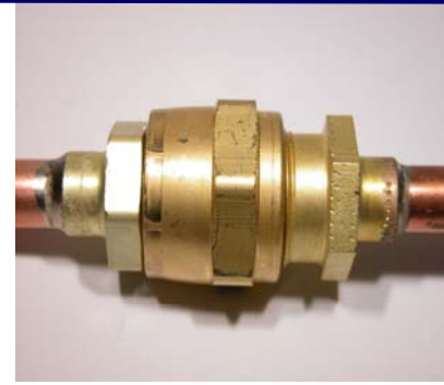
Rotate Swivel Nut One Quarter Turn More After Nut Becomes Tight
